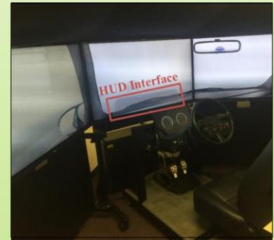
The National Advanced Driving Simulator (NADS MiniSim) was used for the driving simulator experiment.
